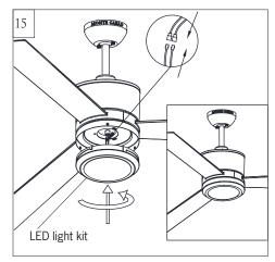
Connect white wire from fan to white wire from LED light kit and then connect blue wire from fan to black wire from LED light kit.
