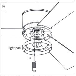
Attach light pan onto the plate on motor, aligning the keyhole slots on the light plate with the preassembled screws on the plate. Twist clockwise till lock. Reinstall the screw removed in step 13. Tighten all screws securely.
