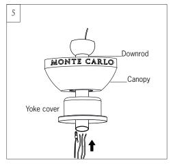
Place downrod over canopy and yoke cover. Thread lead wires and safety cable from motor assembly through downrod.
